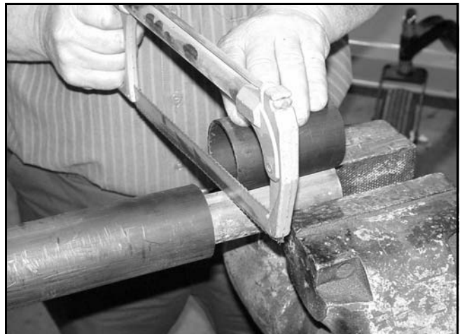
Figure 5. Cut Shaft to Length
